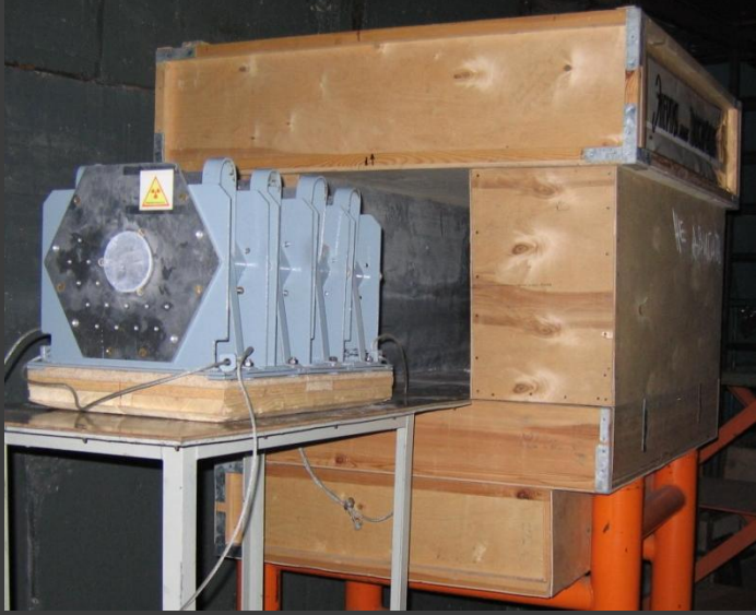
Subcritical assembly + biological shielding
